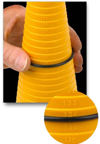
Insert the o-ring to determine the cross section then slide the o-ring down the corresponding side.
