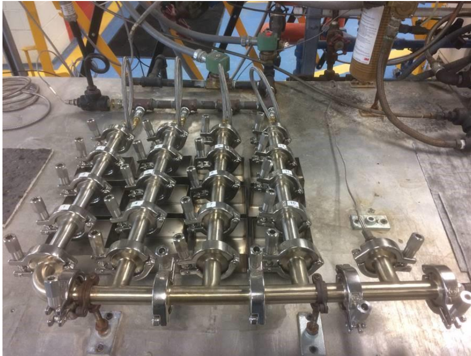
Steam-In-Place test stand for hygienic gaskets
