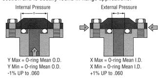
Radial Seals: The squeeze is on the I.D. and O.D. of the o-ring as found in most end cap applications.
