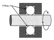
Oscillating: Motion occurs when a shaft rotates backward and forward in a circular arc. Longitudinal motion is usually not significant. Example is a faucet valve stem.
