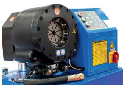
Rubber Fab's hose fabrication team offers 360° radial crimping to our sanitary hose for a positive lock that enables the assembly to be used to the maximum working pressure of the particular hose style and size without fitting pull-off or blowing off.
